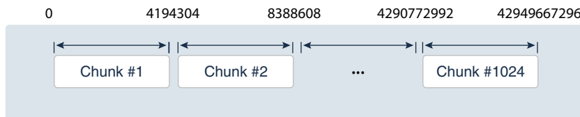
Figure 2-4 Ranges of Hash Values Assigned to Chunks
