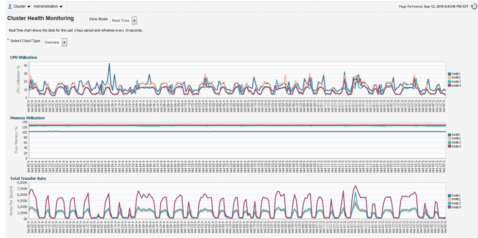
Figure 4-2 Cluster Health Monitoring - Real Time Data
